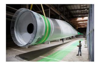
Suzlon SB 63 blade being inspected at Padubidri factory
