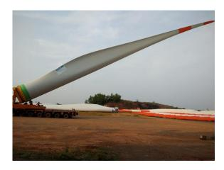
Suzlon SB63 blade mounted on an innovative adapter trailer
